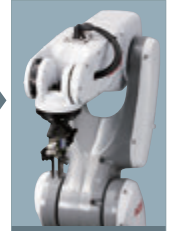
Hollow wrist cables are stored inside wrist
