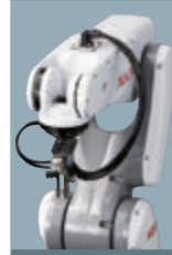
Conventional wrist overhanging cables
